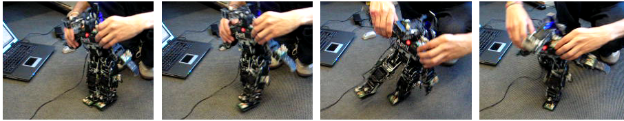
Fig. 7. Transfer of motion pattern to hardware: The 'grounded' real robot shows similar behavior compared to its simulated counterpart, but still needs manual support for walking.
